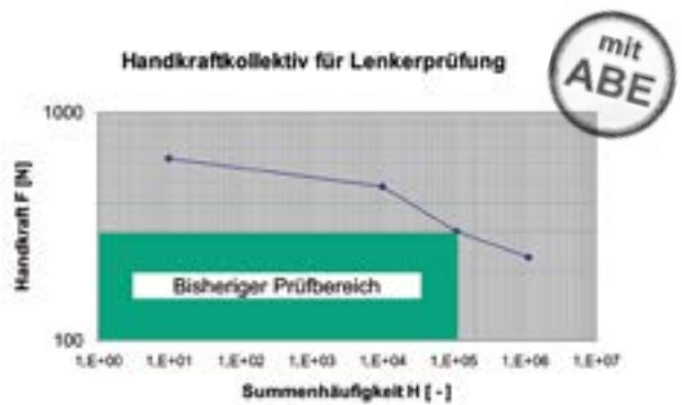
The LSL internal endurance profile is a benchmark for a realistic handlebar test.
