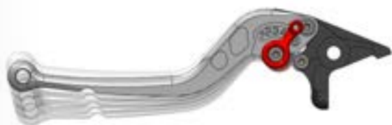
positions of clutch lever: 1-4 closer; 5 app. original position; 6 further
