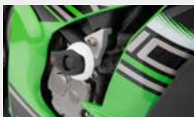
_ 4 Crash Pad®, screwed with adapter plate from page 100
