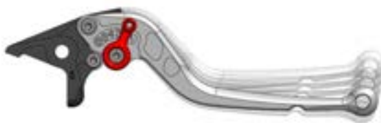
positions of brake lever: 1 closer; 2 app. original position; 3-6 further
